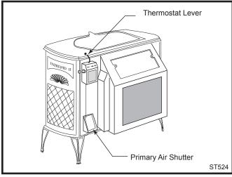
Fig. 29 The primary air shutter must move freely.
